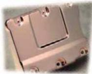
Copper plating can be used for several operations. This soft metal can be applied in thick layers that can be sanded, soldered and polished to a high shine, making its use somewhat like a high build filler paint coat. It may also be used to 'electroform' articles in various ways, and to 'bronze' non-conductive items such as leaves and baby shoes.
